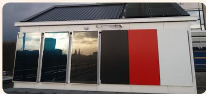
Solar heat collectors based on the usage of NIR absorbing coloured coatings
